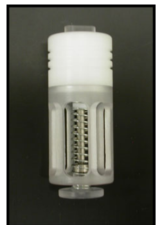
Fig. 1 Photograph of custom-made spring-loaded impactor used for applying SSBMS arrays to skin in vitro and in vivo studies.
